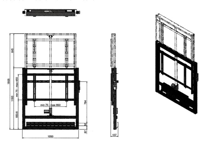
Screen mounting compatibility: supports VESA mounting hole patterns from 75mm to 800mm wide and from 75mm to 400nmm high
