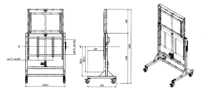
Screen mounting compatibility: supports VESA mounting hole patterns from 75mm to 800mm wide and from 75mm to 400mm high
